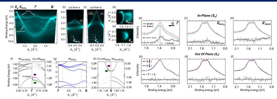
Authors demonstrate a scalable approach to the epitaxial synthesis of  $\operatorname{MoS}_2$  monolayer on a magnetic graphene/Co system. Using spin- and angle-resolved photoemission spectroscopy authors observe a magnetic proximity effect that causes a 20 meV spin-splitting at the  $\overline{\Gamma}$  point and canting of spins at the  $\overline{K}$  point in the valence band toward the in-plane direction of cobalt magnetization.
