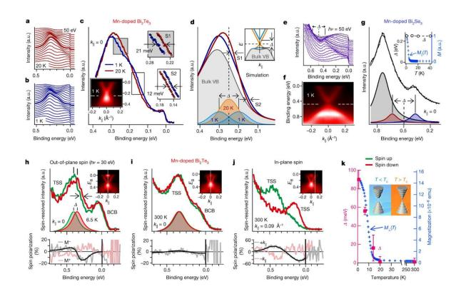
Authors use low-temperature photoelectron spectroscopy to unambiguously reveal the magnetic gap of Mn-doped  ${\rm Bi_2Te_3}$ , which displays ferromagnetic out-of-plane spin texture and opens up only below  ${\rm T_C}$
