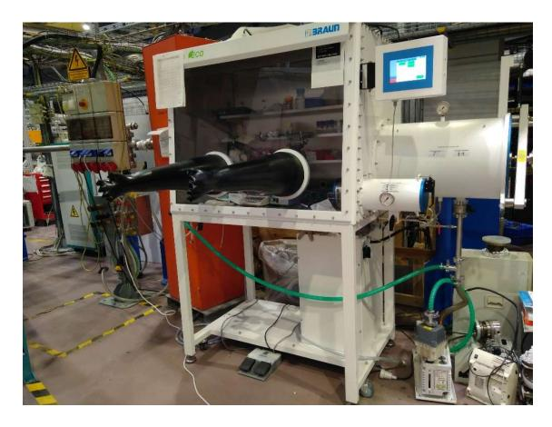
Argon glove box allows transfer of the samples to the experimental station without contact with air
