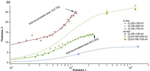
Figure: comparison of the *in situ* and *ex situ* kinetics: (a) and (b) ex situ Ge 3d and Te 4d for a GeTe (111) surface treated with molecular and atomic oxygen; (c) Reaction kinetics for the in situ data obtained at low (green) and high photon flux (brown), ex situ data obtained for molecular oxygen (blue) and in the presence of atomic oxygen (dark yellow).
